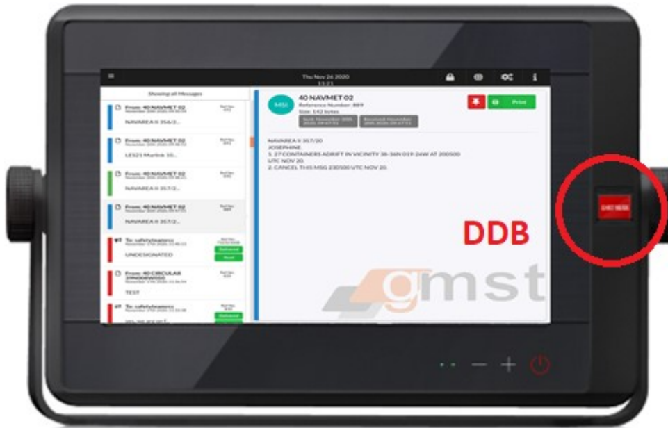
Figure 19 Dedicated Distress Button (DDB)
